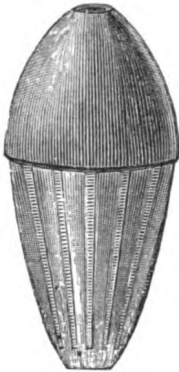
Schenkl projectile, without patch.
